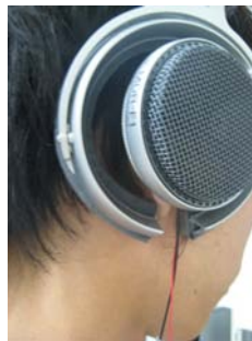
Fig. 7 A listener putting ear-microphones into his entrances of ear canals and wearing open-air headphones
