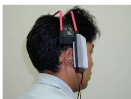
Fig.4 A subject wearing ear-microphones and open-air headphones.
